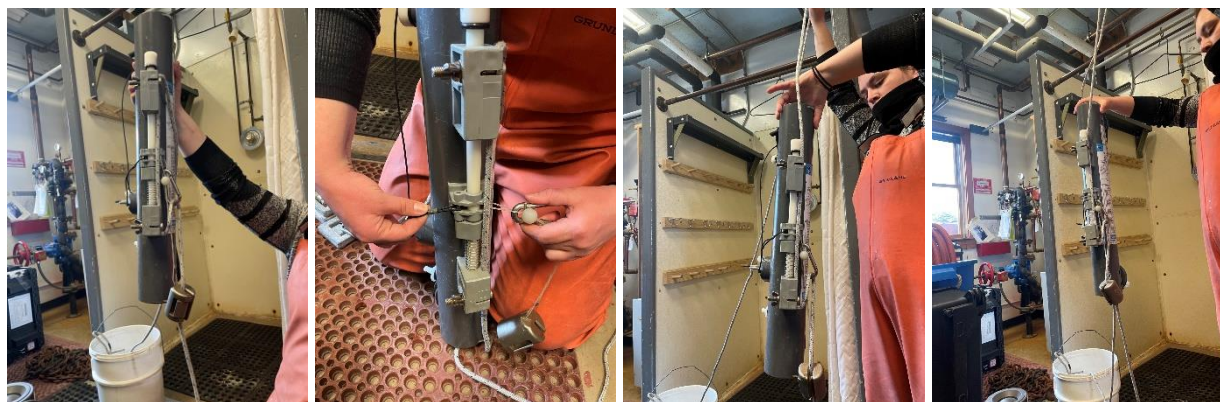
Figure 11- C-045-P (Van Mooy) grantee Shavonna Bent demonstrates the daisy-chain system of Go-Flo bottles for small-boat at-depth water collection at Station E. Image Credit: Maya Thomas
