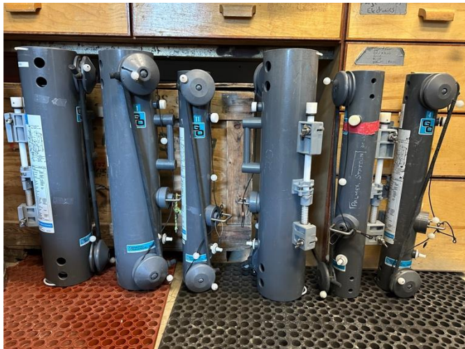
Figure 8- Go-Flo Bottles of various sizes used for manual sampling at Station E from zodiacs. Image credit: Sneha Sivaram
