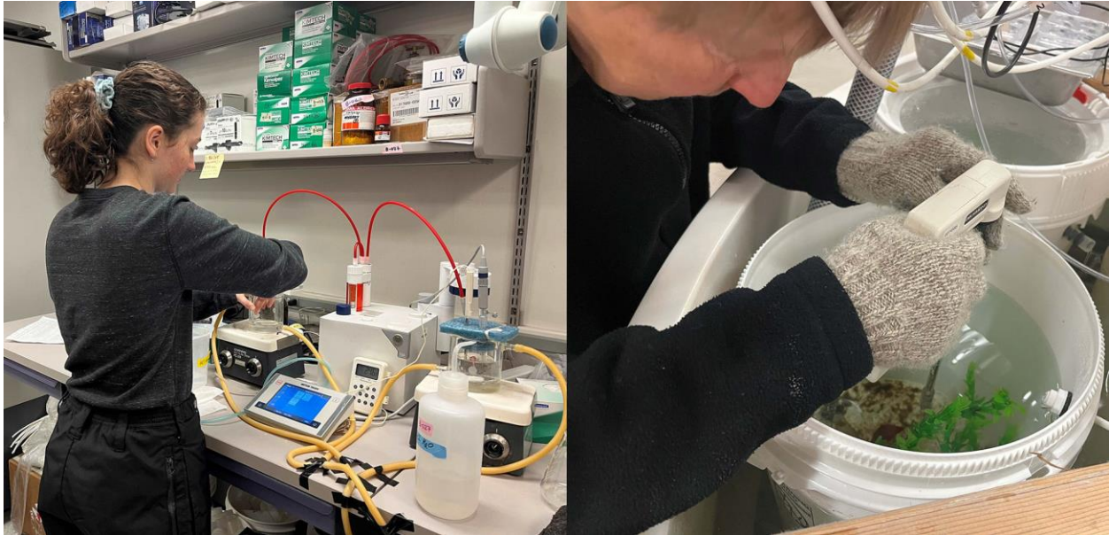
Figure 4- Left: The titrator used to determine seawater alkalinity. Right: removing amphipod molts and dead amphipods, if any, from an experimental bucket.
