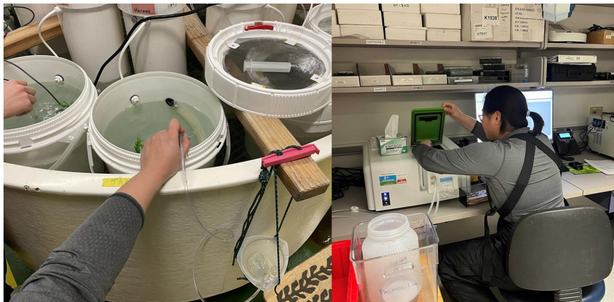
Figure 3- Left: Water being siphoned out of an experimental bucket for seawater chemical analysis. In the bucket to the left of the image, the pH is being measured using a pH probe (done with each bucket each day) and the bucket temperature is also being measured. Right: Spectrophotometric measurement of pH.
