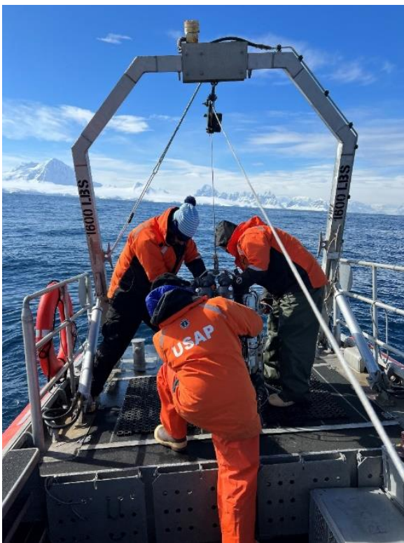
Figure 17: Left: Mackenzie Curtice (C-045-P), Sneha Sivaram (C-019-P), and Lance Roth (ASC Instrument Technician) prepare to deploy the CTD rosette into the water at Station E to collect both science groups' water for the day. Photo credit Matt Cabell. Right: C-045-P (Van Mooy) grantee Mackenzie Curtice prepares to filter the seawater collected from Station E. Photo credit Dr. David Fields.
