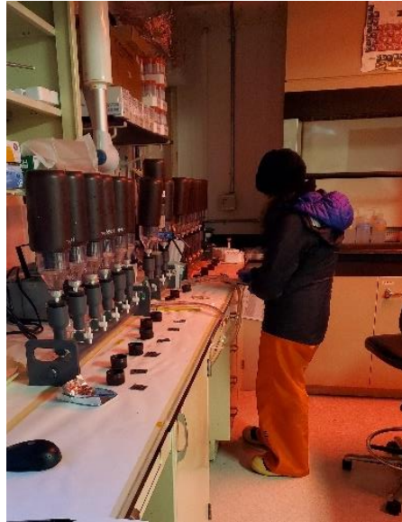
Figure 12: : Sneha records metadata on log sheets as bottles of water collected from Station E filter on vacuum filtration rigs (photo credit Malarie O'Brien)
