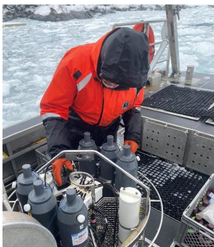
Figure 15: C-045 (Van Mooy) grantee Mackenzie Curtice checks the hardware components of the CTD Rosette onboard Hadar as the LTER group prepares to head out to Station E. (Photo credit Carlyn Scott)
