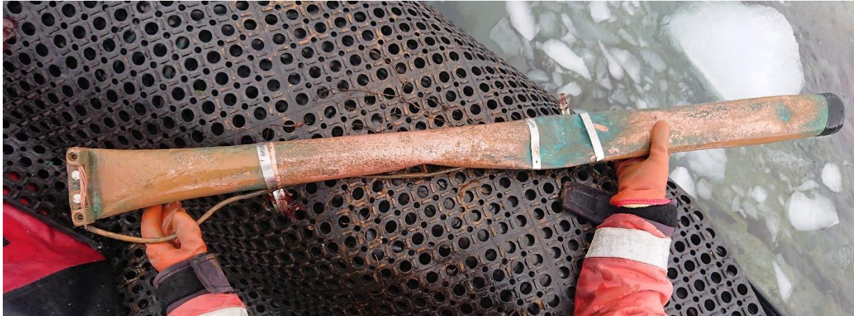
Grounding cable terminus before returning to the bottom of Hero Inlet. Image Credit: Randy Jones
