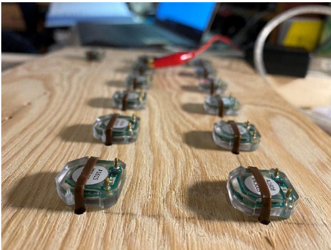
GLS tags being calibrated for giant petrel deployment. Image Credit: Cimino group
