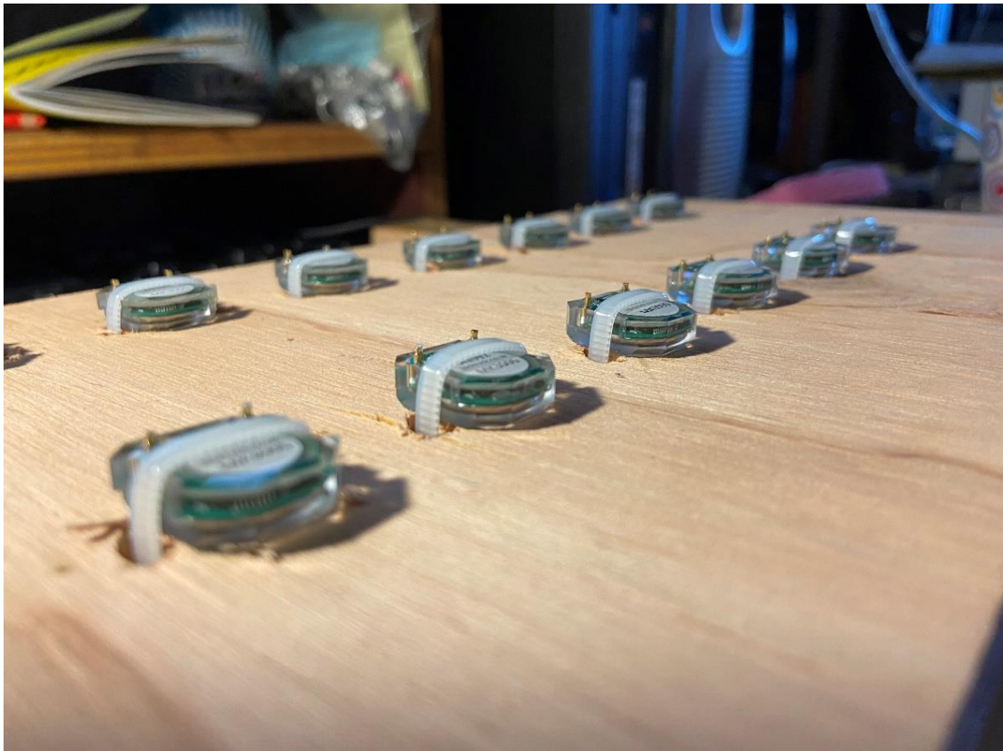
GLS tags prior to deployment on Giant Petrels. Image Credit: Fraser group
