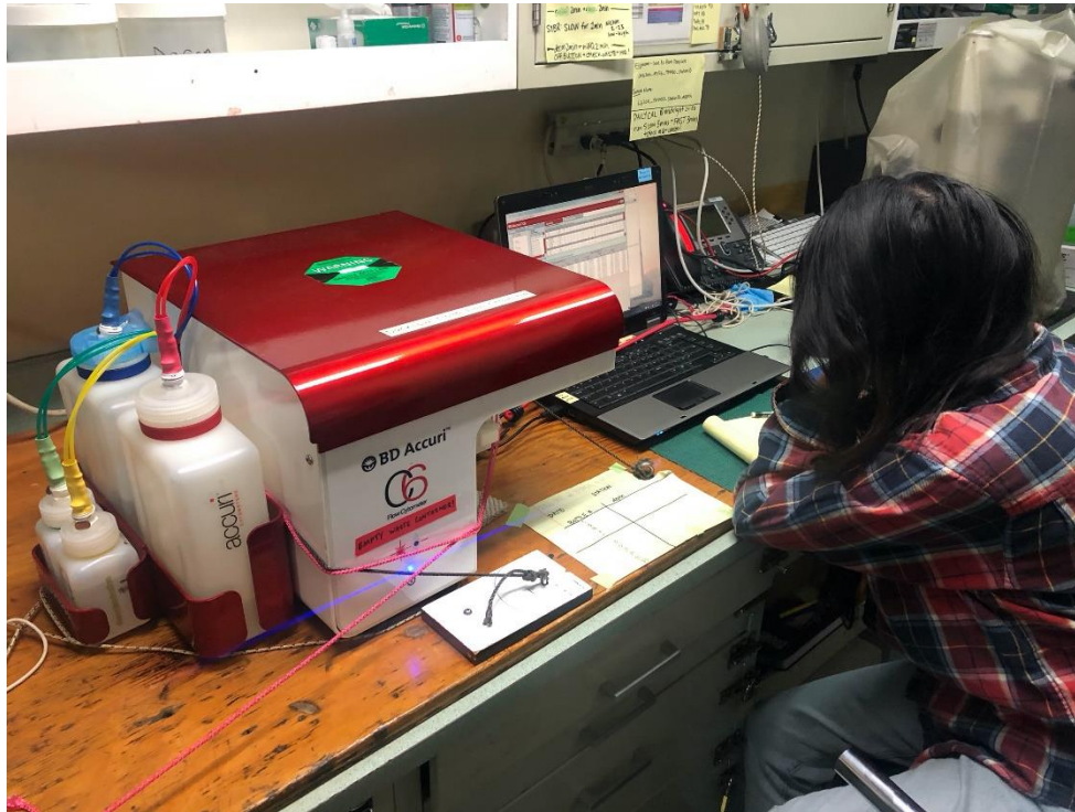
Ducklow lab member, Natalia Erazo, processing flow cytometry samples on the LTER cruise, 2 February 2020. While on the boat, the Accuri flow cytometer must be tied down with rope and bungee cords to prevent its movement in rocky seas. Image credit: Ducklow group
