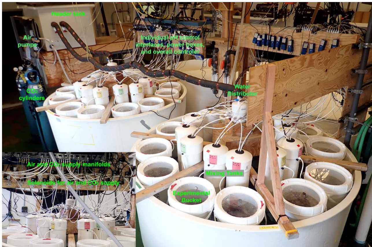
Fig. 3 – B-027-P main ocean acidification experiment. See text for explanation of labels. The inset in lower left shows the back of the plywood panel labeled “Individual pH control interfaces...” on the main image.
