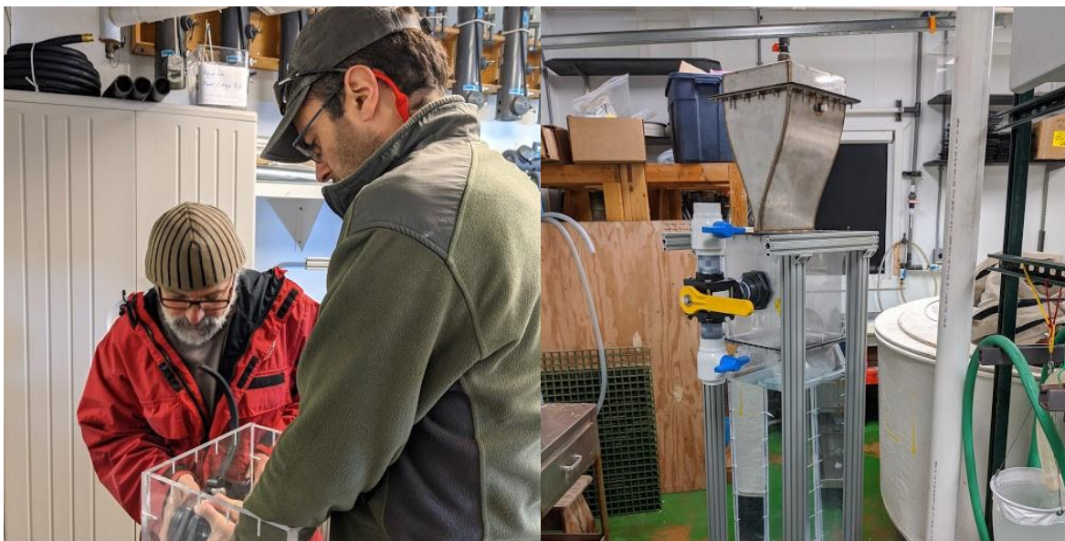
Fig. 2 – David Fields and Laboratory Supervisor, Randy Jones, assembling the vertical flume (left) and the assembled flume (right).
