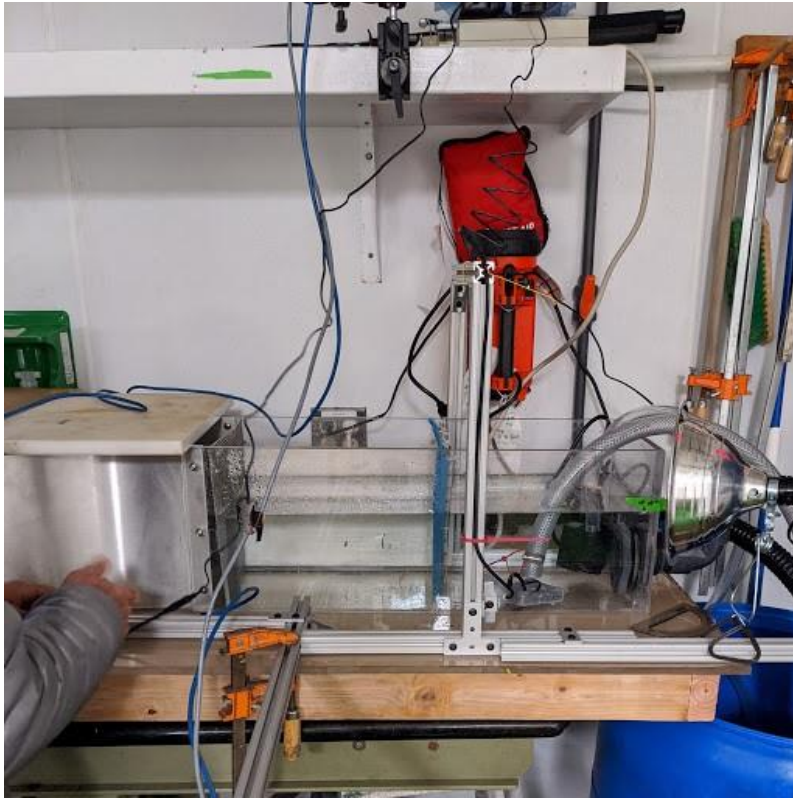
Fig. 5 – Horizontal flume showing working section, camera and light set up
