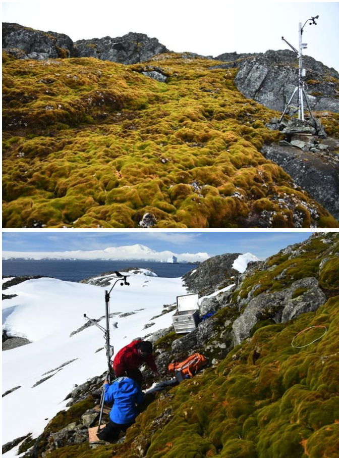
Fig. 15 – Photos of two microclimate stations with 5 sensors for Photosynthetically Active Radiation (PAR), air temperature and relative humidity, wind directions and speed, soil temperature, and soil moisture. Top: Norsel Point (installed on 17 January 2019); Bottom: Joubin Island #4 (installed on 22 January 2019; Dulcinea Groff and Zhengyu Xia working on stabilizing the tripod). Image Credit: Yu group.
