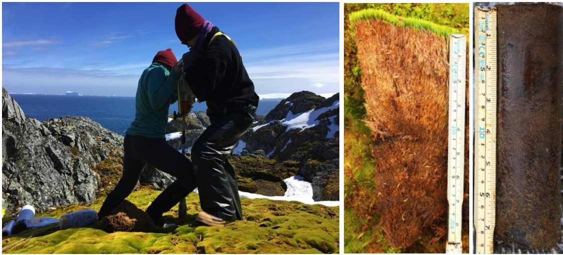
Fig. 17 – Peat coring of a large peatbank on Upper Green Valley on Litchfield Island. Left: Peat coring using a specially-built small-diameter permafrost corer to minimize damage to sensitive Antarctic peatbank ecosystems by Dulcinea Groff and Zhengyu Xia; Middle: Surface monolith collected using a bread knife; and Right: Frozen section of the core 100 cm below the surface (Image Credit: Yu group).
