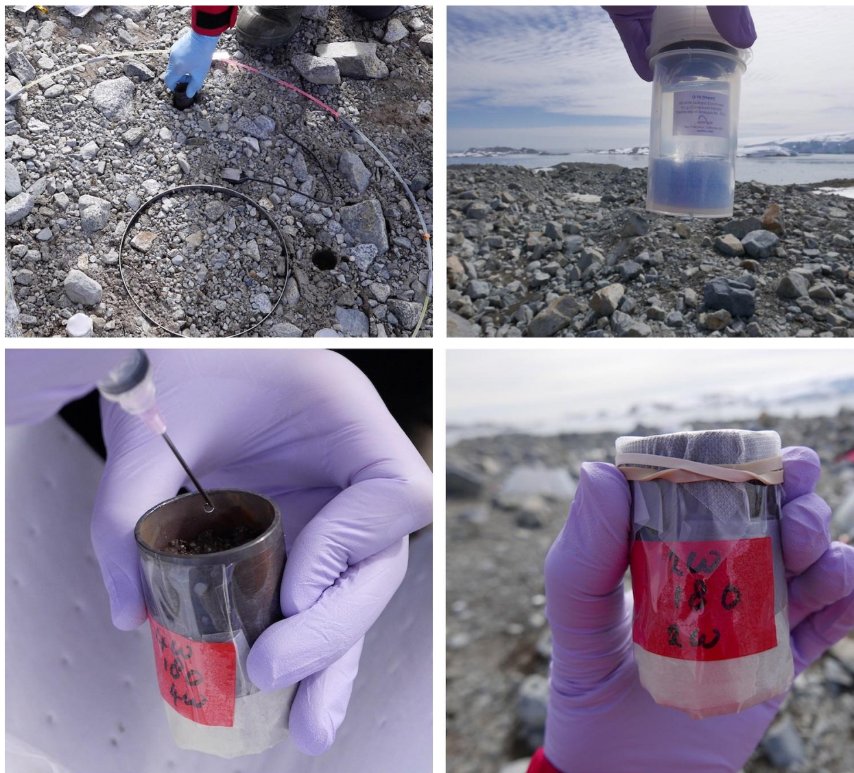
Fig. 3 – Field incubation of intact soil cores in warmed and control plots. Intact soil samples are inside the stainless steel cores. The soils inside the cores receive either pure water (containing mostly oxygen-16) or heavy water (containing mostly oxygen-18). Microbes that are growing incorporate oxygen into their DNA, so microbes receiving heavy water will have heavier DNA. The density of microbial DNA will be assessed at Northern Arizona University, and sequencing will reveal who are heavier.
