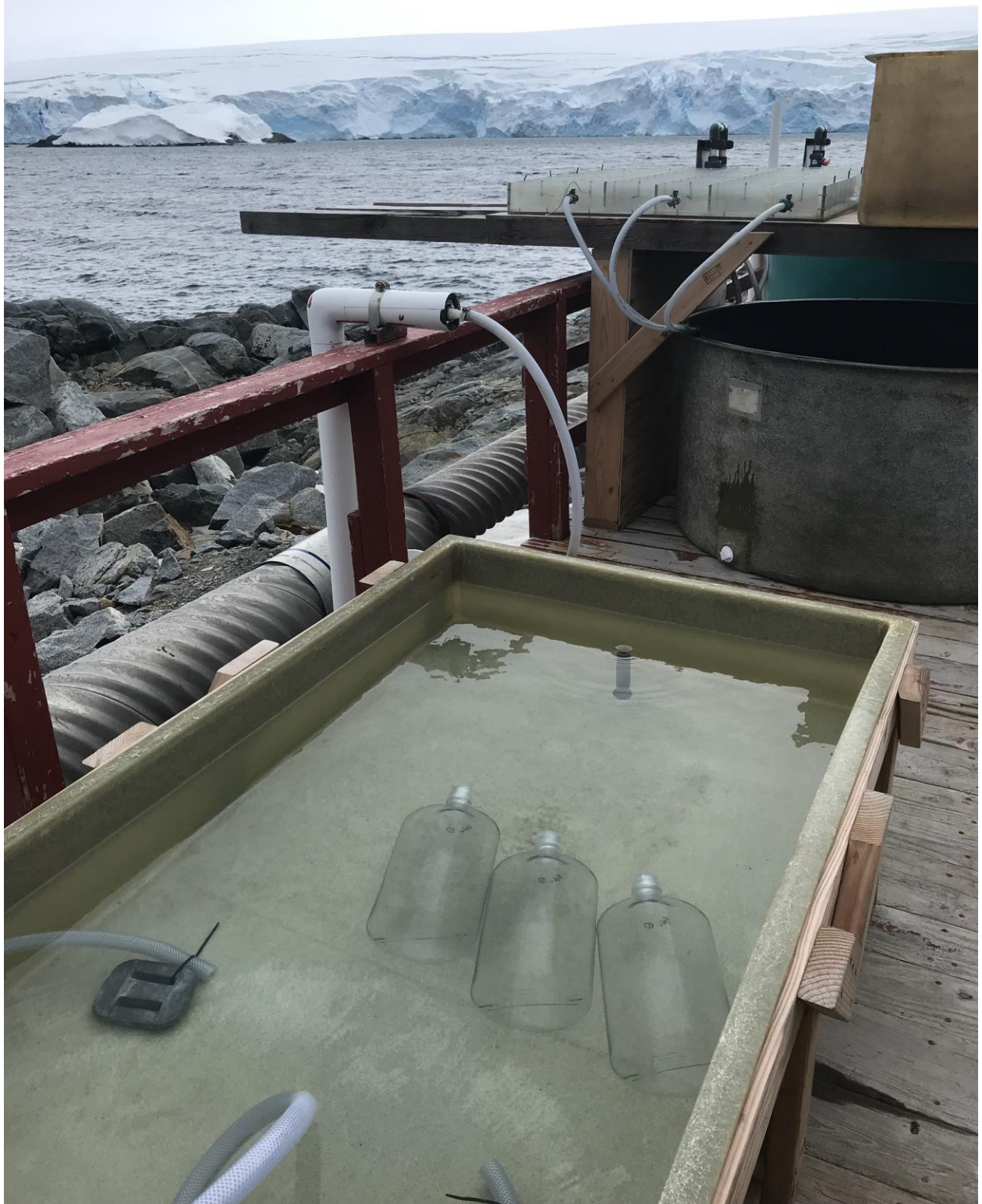
Fig. 14 – ^{15}\text{N}_2 incubation experiment in an outdoor cascade tank (Image credit: Shuai Gu).
