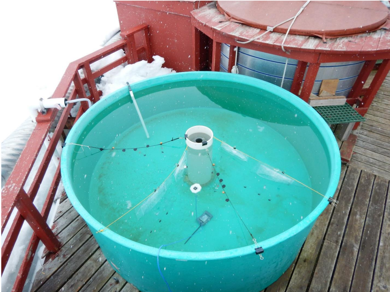
Fig. 3 – Various analytical methods were used to measure reactive oxygen species production and incident light fluxes in an open-air aquarium on the Palmer Station aquarium deck (Image Credit: Van Mooy group).
