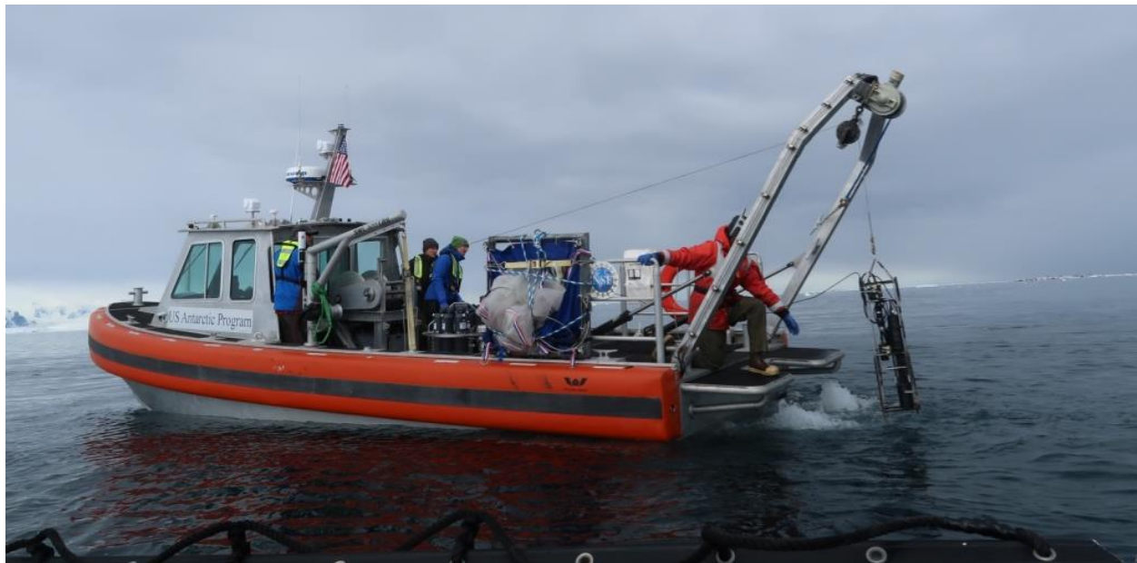
Fig. 4 – Deploying the AC9 optics cage off the stern of RHIB Rigil (Image Credit: Keri Nelson).
