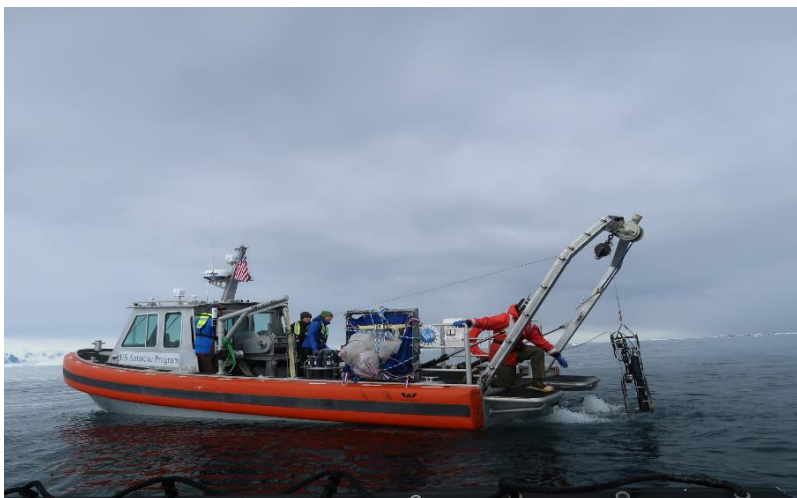
Fig. 11 – Deploying the AC-9 for the C-019 (Schofield) team, using the winch in a similar manner to how we would deploy our beloved CTD. (Image Credit: Keri Nelson)
