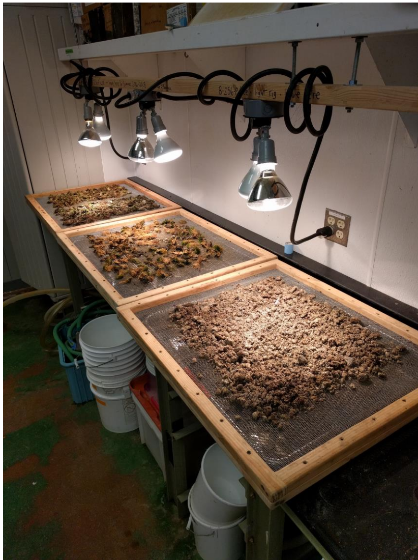
In the Aquarium, vegetation and soil samples dry under incandescent lamps in setups designed to extract Belgica antarctica from the samples and into the trays below. Image Credit: Randy Jones
