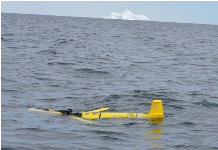
Fig. 7 –The autonomous underwater glider, RU24, at deployment.
