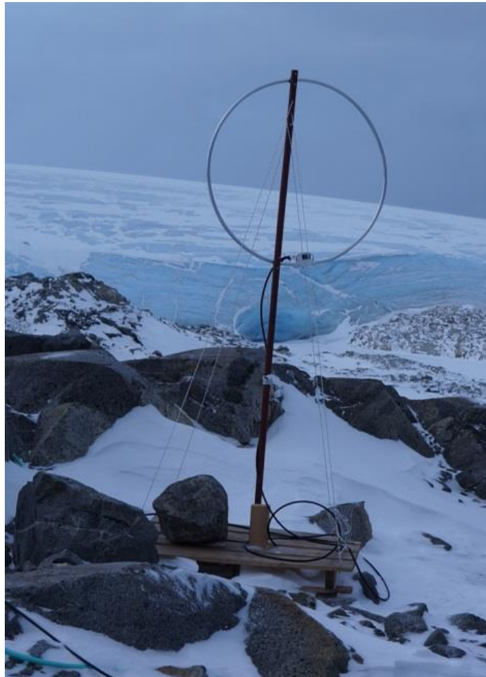
Figure 3. HF receive antenna installed behind Terra Lab building.
