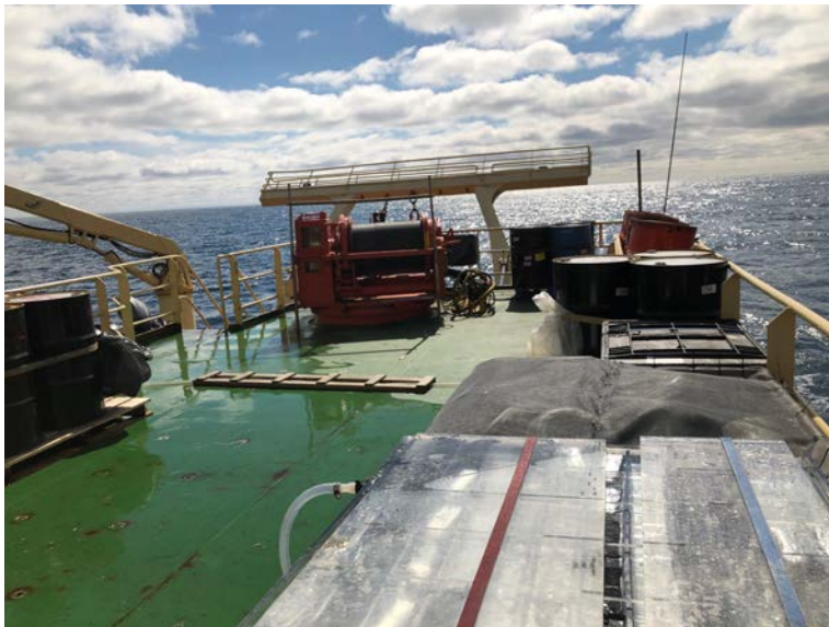
Figure 5. The phytoplankton productivity incubator on the 01-deck in the foreground. Samples screened to different light values are visible within the deckboard unit on our first sunny day of the cruise.
