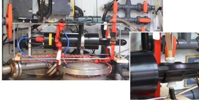
Figure 1. A Sequoia Scientific LISST-HOLO holographic camera was plumbed into the ship's seawater delivery system for the transit across the Drake Passage. The flow was sampled before bubble removal and after the flow passed through a coarse mesh that prevented large particles from making it to the camera.
