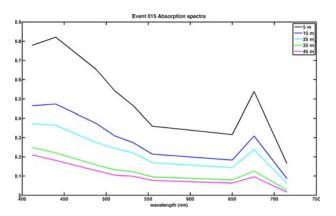
Figure 4. Spectral absorption data collected by the AC-9 instrument. The data clearly shows the strong soret peaks associated with chlorophyll and carotneoids. At depth, the steeper exponential rise relative and relative decline in carotenoid absorption suggest the relative increase in colored dissolved organic matter and detritus.
