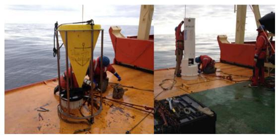
*Figure 3.* Pictures of both sediment traps before being redeployed again to sample until next years cruise.
