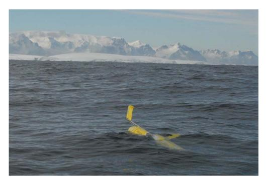
**Figure 1.** Webb-Slocum Rutgers Glider during deployment on 07 January off Palmer Station.
