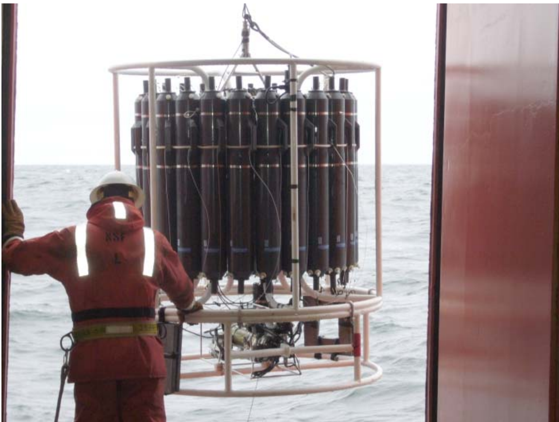
Figure 1. MT Greg Buikema recovers the CTD-Rosette through the Baltic Room door at Station 300.060 on 21 January.
