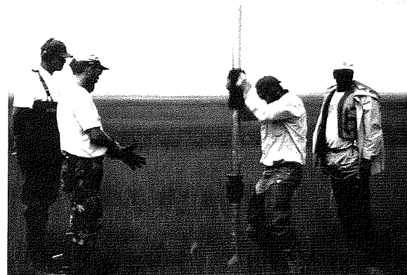
Figure 2. Installing Sedimentation Erosion Table pipe in Spartina patens at Nauset Marsh, Wellfleet, Cape Cod National Seashore MA. (Photo by Charles Roman, USGS)
