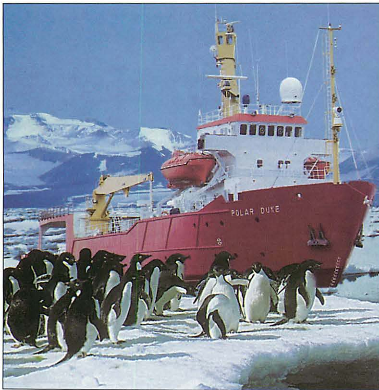
Figure 2: The R/V Polar Duke is an ice-strengthened vessel with accommodations for 26 scientists. Diesel propulsion and thrusters fore and aft provide excellent maneuverability and station keeping. Photo by Rieber Shipping A/S.
