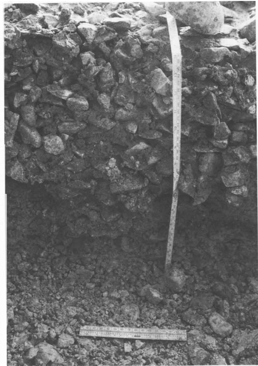
Fig. 3. Profile of Test Pit 1 at the modern Adélie penguin colony on Litchfield Island. Ornithogenic soils, comprised of pebbles and dark organic sediments, extended to a depth of 30 cm before greyish, finer-grained sediments and angular gravel were reached. Scales in centimetres.
