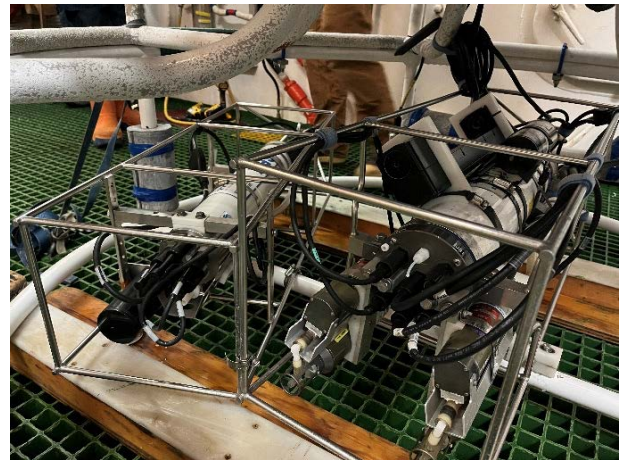
Figure 3. SBE19plus from the British Antarctic Survey that attached to our rosette next to our SBE9plus.
