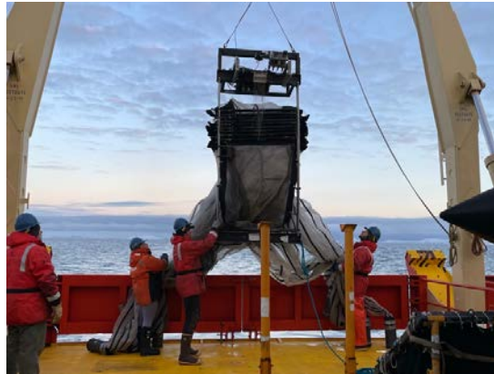
Figure 10. Deploying the MOCNESS for a night tow. This tow fished to 500 m, and collected zooplankton in 8 discrete depth intervals. Photo by Debbie Steinberg.
