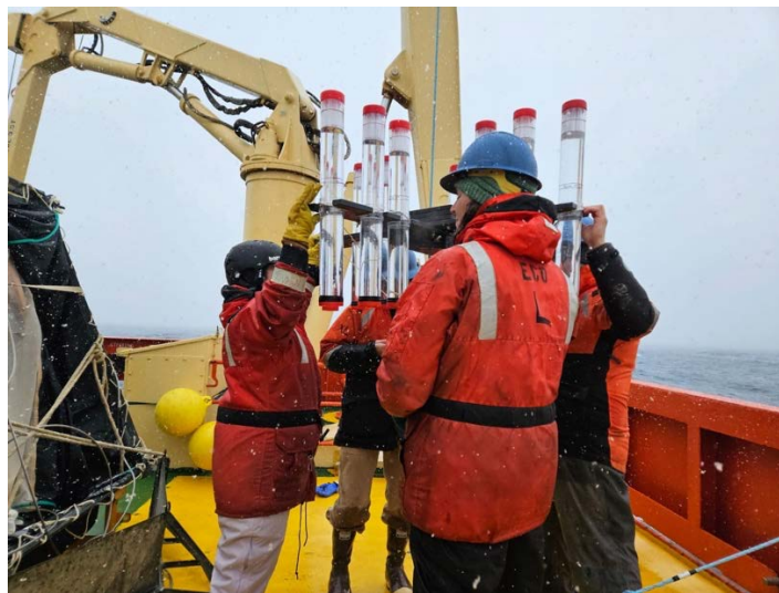
Figure 4. Recovering the sediment trap (Particle Interceptor Trap, PIT). Each cross frame holds nine tubes into which sinking organic particles are collected, and each sediment trap array collects these samples at 3 depths. The vertical array is attached to a surface float and drifts freely but with a satellite tracker so its position can be monitored. Photo by Laura Motta.
