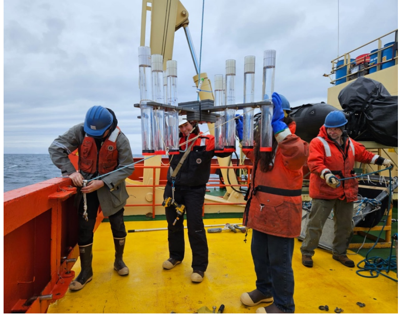
Figure 5. Deployment of drifting sediment trap at Process Study 1 in the Palmer Deep; photo by Laura Mota
