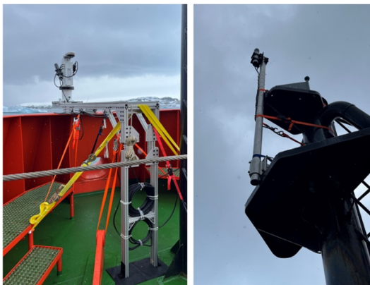
Figure 7. HyperSAS mounted on ship’s bow (left) and sensor on the mast (right).
