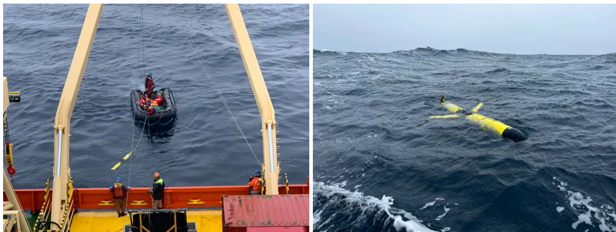
Figure 3: NOAA Glider AMLR05 is deployed from the N.B. Palmer on November 25th, 2021.
