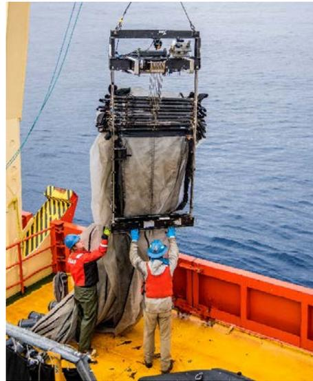
**Figure 6. Deploying the MOCNESS system from the back deck of the Gould during week 4.**
