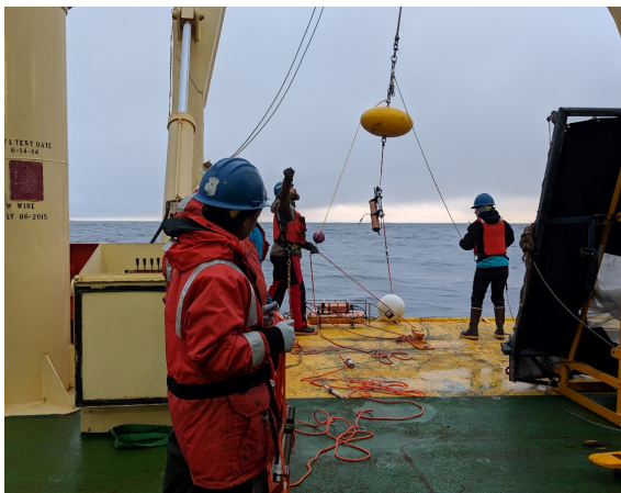
Figure 2. Scientists stay out of the yellow zone while MT Josh Mitchell and MLT Diane Hutt use the stern A-frame to lift the heavy yellow EF-33 top float off the ship. In the air is the SeapHOx, which will monitor pH and oxygen. On the deck is the CO 2 Pro, which monitors carbon dioxide throughout the year.
