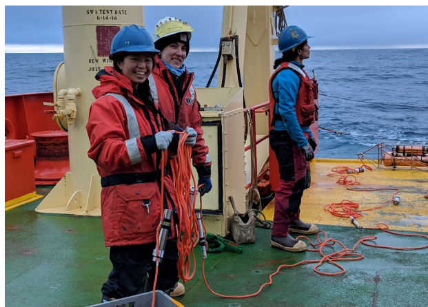
Figure 3. Rebecca Trinh (left), Naomi Manahan (right), and ET Adina Scott prepare to hand line to the people working in the yellow zone. The metal instrument hanging from the line in Rebecca's hand is a temperature/pressure sensor that sits at a specific depth in the water column.
