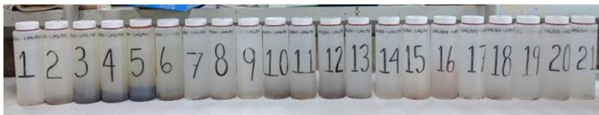
Figure 4. Sediment trap bottles lined up in order of sampling. Bottle 1 began collecting sinking particles on February 4, 2018. Cups that show high flux (indicated by high particle volume) are bottles 4 and 5, which collected during the months of March and April 2018, respectively.
