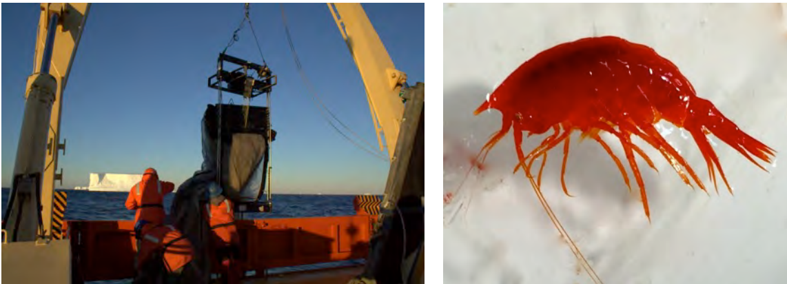
Figure 6. Deep MOCNESS tow. Left, deploying the MOCNESS; right, a deep-sea amphipod, likely Cyphochyrus sp., collected between 750-1000m. (Photo credits-N. Shelton and D. Steinberg, respectively)
