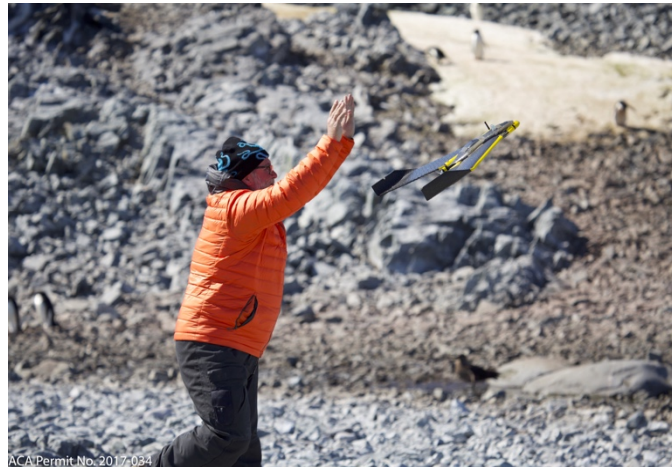
Figure 11. The eBee is hand-launched for flights over penguin colonies at Avian Island, Western Antarctic Peninsula
