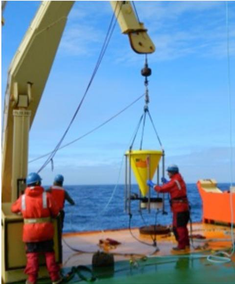
**Figure 4.** Sediment trap deployment.
