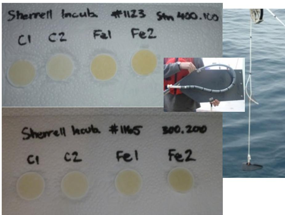
**Figure 10.** Fe-addition incubation results for stations 400.100 and 300.200. Water was collected using the trace metal towfish (inset) and incubated in duplicate control (C) and +Fe (Fe) for 5-6 days. The more intensely pigmented +Fe filters suggest that Fe-stress or limitation was structuring the phytoplankton assemblage at these stations. Full pigment analyses using HPLC, and macronutrient concentrations at time of harvest, will tell a more complete story.
