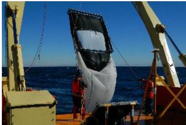
**Figure 8.** Deploying the large, 2-m square Metro net used for sampling krill and other macrozooplankton on an unusually sunny day this week.
