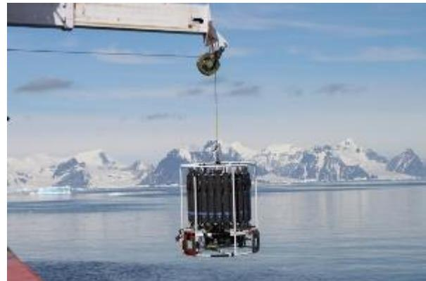
**Figure 2.** CTD cast in Ryder Bay near the British Antarctic Survey (BAS) Rothera Base.
