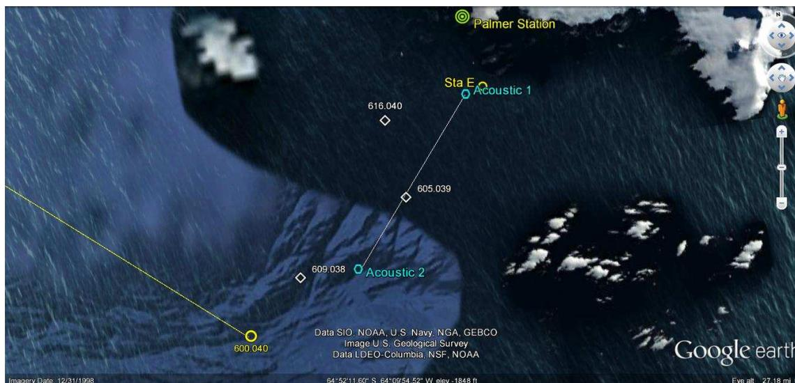
**Figure 2.** Map of stations occupied during LTER cruise Process Study 1. Shaded bathymetry in the lower left shows the Palmer Deep submarine canyon. LTER grid station 600.040 (bottom left) is in the deepest part of the Palmer Deep (1200 m). Diamonds show CTD stations occupied on the sides of the canyon during Jan. 5-8. Palmer Station is near top of the diagram.
