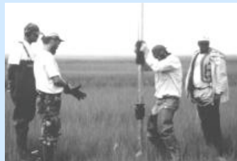
Installing Sedimentation Erosion Table pipe in Spartina patens at Nauset Marsh, Wellfleet, Cape Cod
